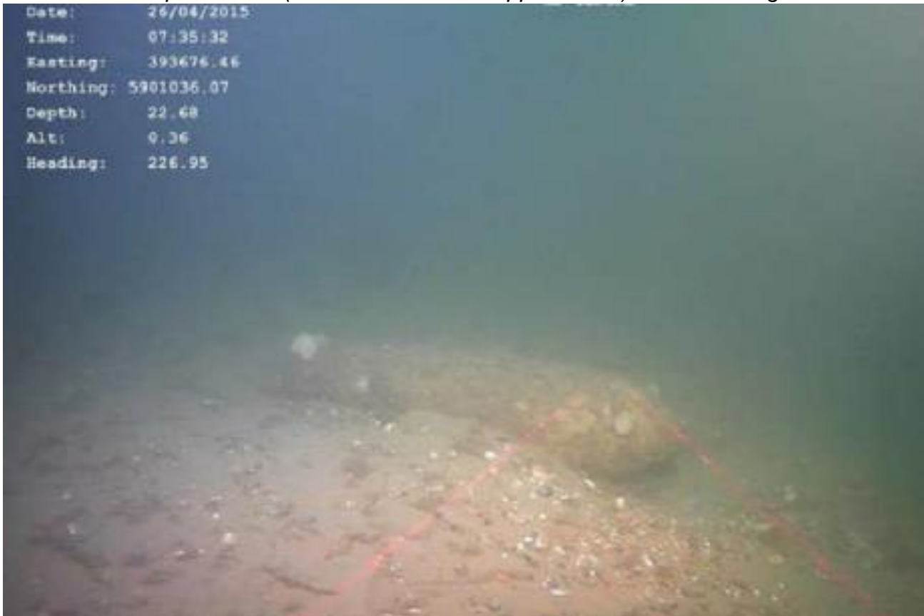
Plate 5-4: Example of UXO (500lb German air dropped bomb) from the Dudgeon OWF
